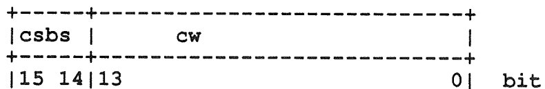
Fig. 13.1 The s_dtgreq and s_streq sub-fields format
