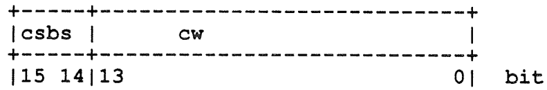
Fig. 6.3.1 The rb.ass[n].stream and rb.ass[n].dgram formats
