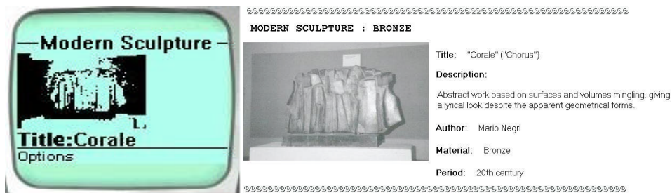
Figure 3.6. Same task (accessing a work of art), different domain concepts: a Functional Core Adaptor level adaptation. On the left, only the first-class attributes of a work of art are displayed for WAP-enabled phones. On the right, users have access to all of the attributes available about works of art.
