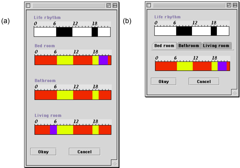
Figure 9: a) Large screen: 24-hour temperature settings are available at a glance for every room of the house. b) Small screen: 24-hour temperature settings are displayed for a single room at a time.
