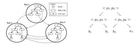
Fig. 1. The GHT\* network (a) and an example of Address Search Tree (b)
