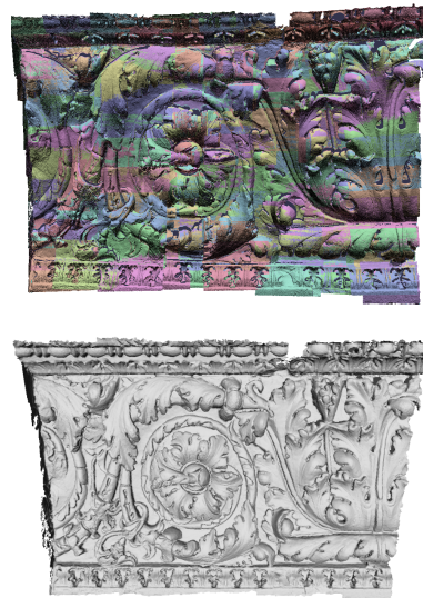
Fig. 9. The coarse alignment of a portion of the archway of S. Ranieri’s door, Pisa Cathedral ( up ). The final model after ICP and global alignment ( down ).
