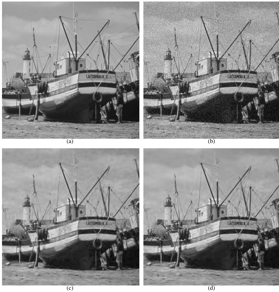
Fig. 3. Results of various denoising methods: (a) Original image; (b) Noisy image ( \sigma = 25 ); (c) Subband adaptive algorithm ( PSNR = 28.95 dB); (d) Local adaptive algorithm ( PSNR = 29.21 dB)
