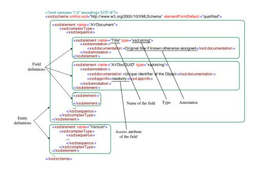
Figure 3. Illustration of the schema definition of the Metadata Model.
