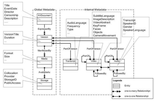
Figure 1. Schematic representation of the ECHO Metadata Model.
