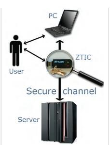
Figure 1: The secure channel is opened between the (bank's) server and the ZTIC. The user communicates as usual with the server via a PC.
