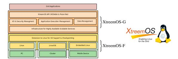
Figure 1. Layering of the XtreemOS architecture.
