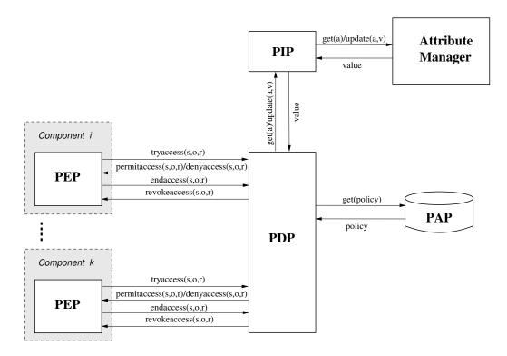
Figure 3: Architecture of the Authorization System.
