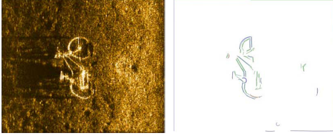
Figure 4: ELSD curve detection result on a sonar map Imagery from jwfishers.com
