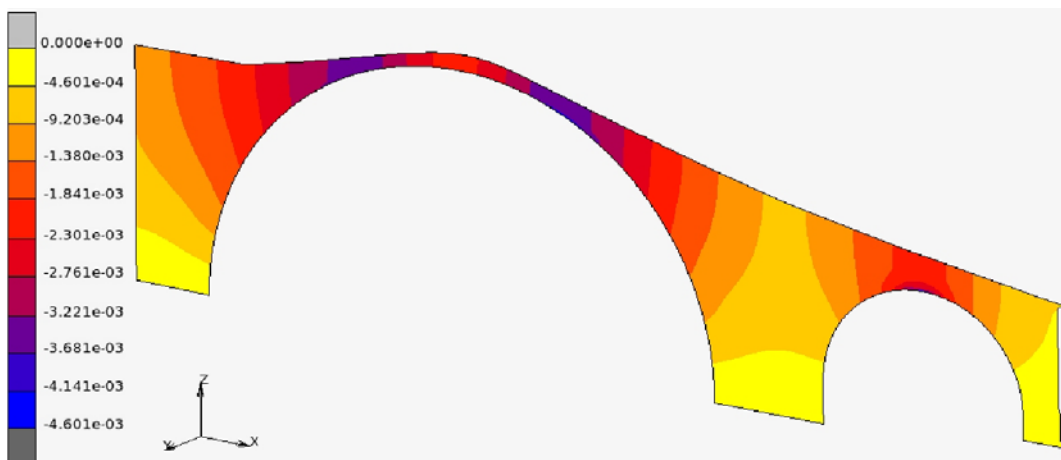
Figure 7. Model 2: map of z - displacements [m] - main arch magnified.
