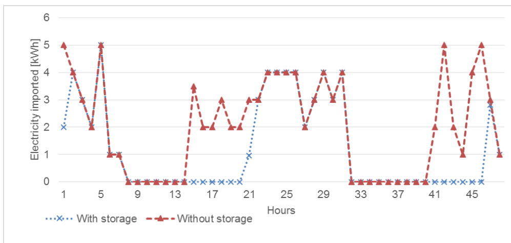
11 12 Fig. 10 - Energy required from grid with PV Generation alone and with a combination of PV-Generation and Storage
