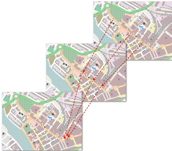
Fig. 21: Because of delays caused by boarding passengers the headway between buses is successively eroded over time until the buses are essentially ‘clumped’ together.
