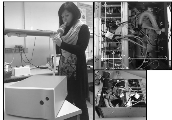
Figure 2: Final configuration of the first prototype of the Wize Sniffer.
