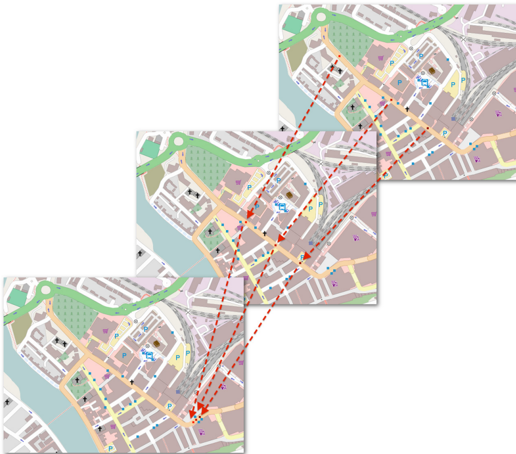
Figure 10: Because of delays caused by boarding passengers the headway between buses is successively eroded over time until the buses are essentially working as a conglomerate.
