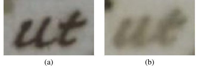
Fig. 1. Example of the typical smearing of the ink that seeps through the paper fiber: (a) foreground text; (b) corresponding bleed-through text.
