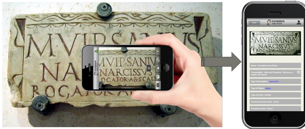
Fig. 1. Example of an application that enables a user to get information about a visible inscription by taking a photo with a mobile device. The application uses a visual search engine to retrieve the photographed object from a database of inscriptions and provides the related information to the user. In the depicted example, the provided information are the transcription of the inscription ( M(arcus) Vipsanius / Narcissus, / rogator ab scaena. ), the type of the inscription ( sepulchralis ), the type of the object ( tabula ), and its present location (Roma), just to cite some.
