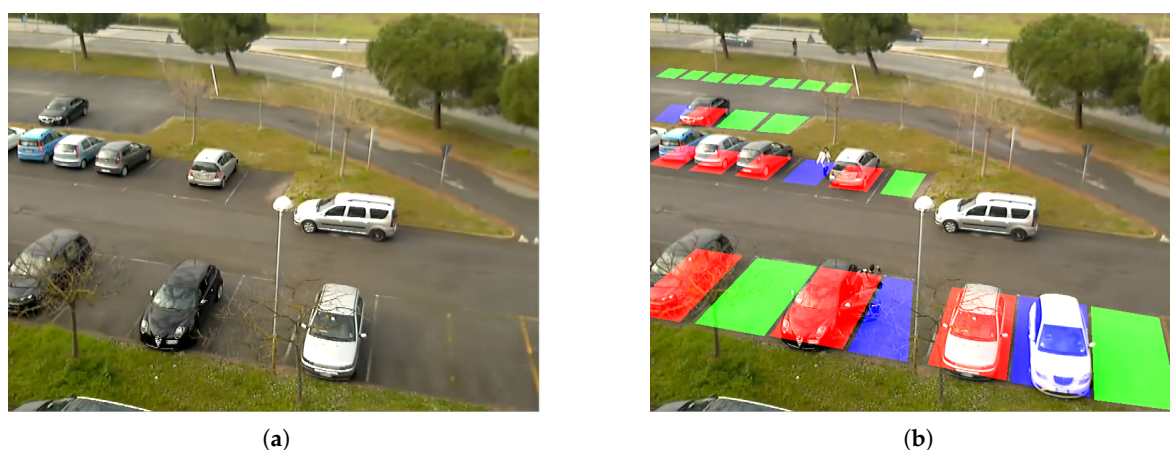
Figure 6. Example of parking lot analysis: background model at time t (a) and real-time output at time t (b).
