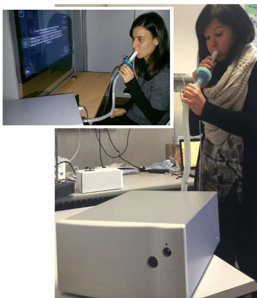
Figure 5. Final configuration of the Wise Sniffer. On the left, the WS is used a Wise Mirror tool. On the right, it is used in a stand-alone configuration.
