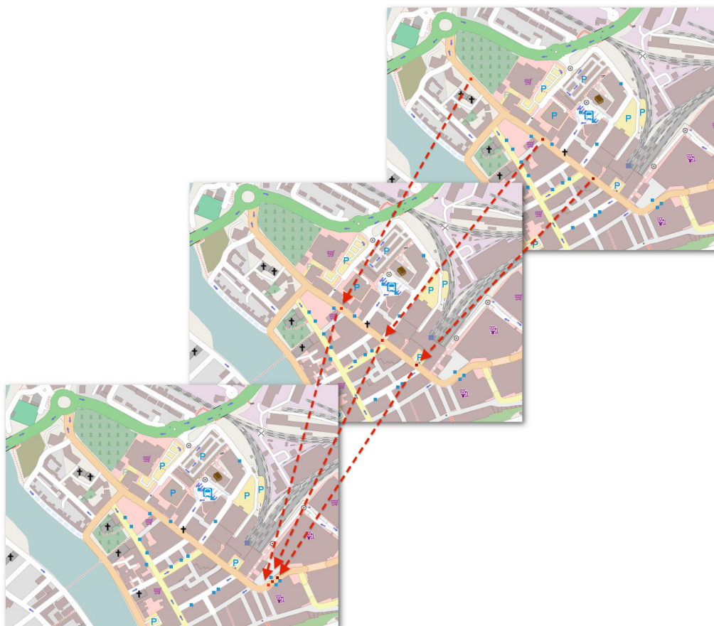
Figure 24: Because of delays caused by boarding passengers the headway between buses is successively eroded over time until the buses are essentially ‘clumped’ together. The successive time frames run from top to bottom.
