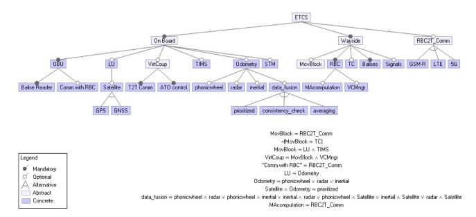
Figure 2: A feature model for ERTMS/ETCS systems (created with FeatureIDE [15])
