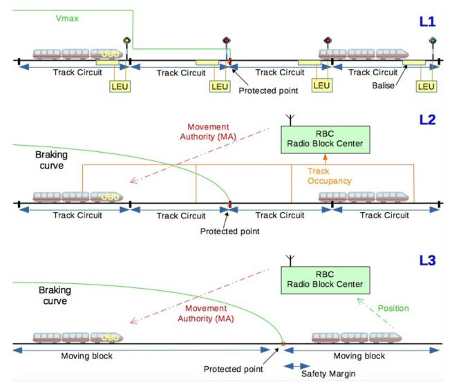
Figure 1: ERTMS/ETCS levels L1, L2, and L3
