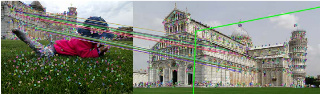
Figure 2.2: Images compared by matching their local features and searching for a geometric transformation that can associate the regions of both images. In this example, ORB [221] features and the RANSAC [102] fitting model were used. Note that no features are localized in flat regions (like the sky) of the images because features need to be distinctive. In the right-hand figure, the green lines are two of the four edges of a bounding box (estimated via RANSAC) delimiting the region of the figure that matches the left-hand figure. The other two edges of the bounding box fall outside the image.
