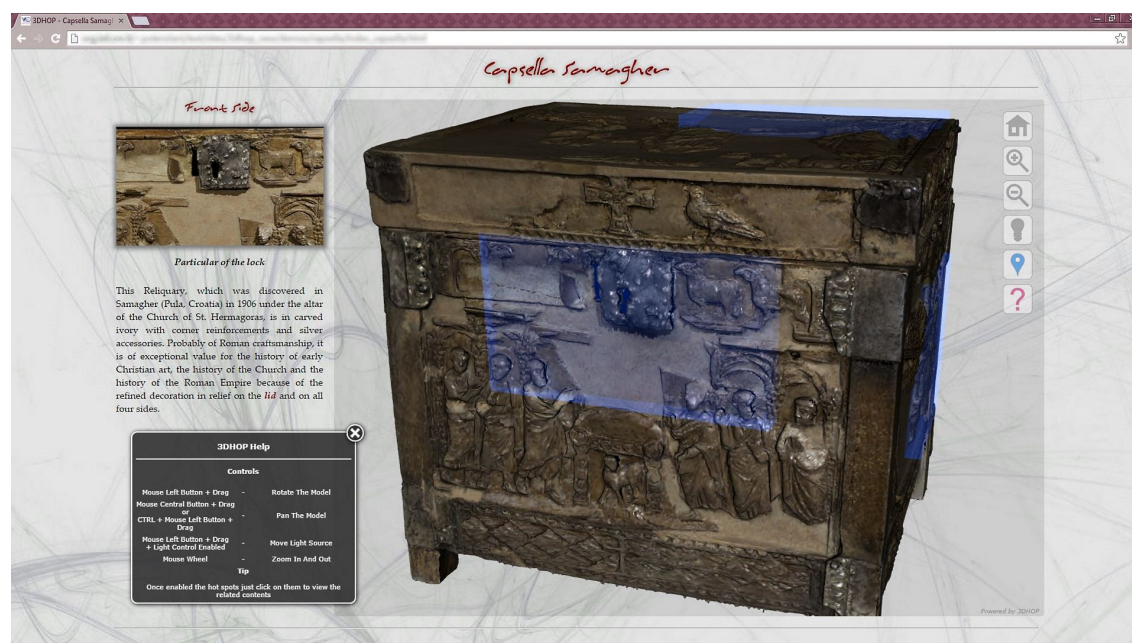
Figure 3.6: The Capsella Samagher viewer: in this 3DHOP [Vis14a] example, the antique reliquary and its lid are presented with hot-spots (light-blue regions). The hot-spots, when picked, centers the view over the hot-spot area and show the corresponding descriptive content (images and text) in the left-most part of the webpage.
