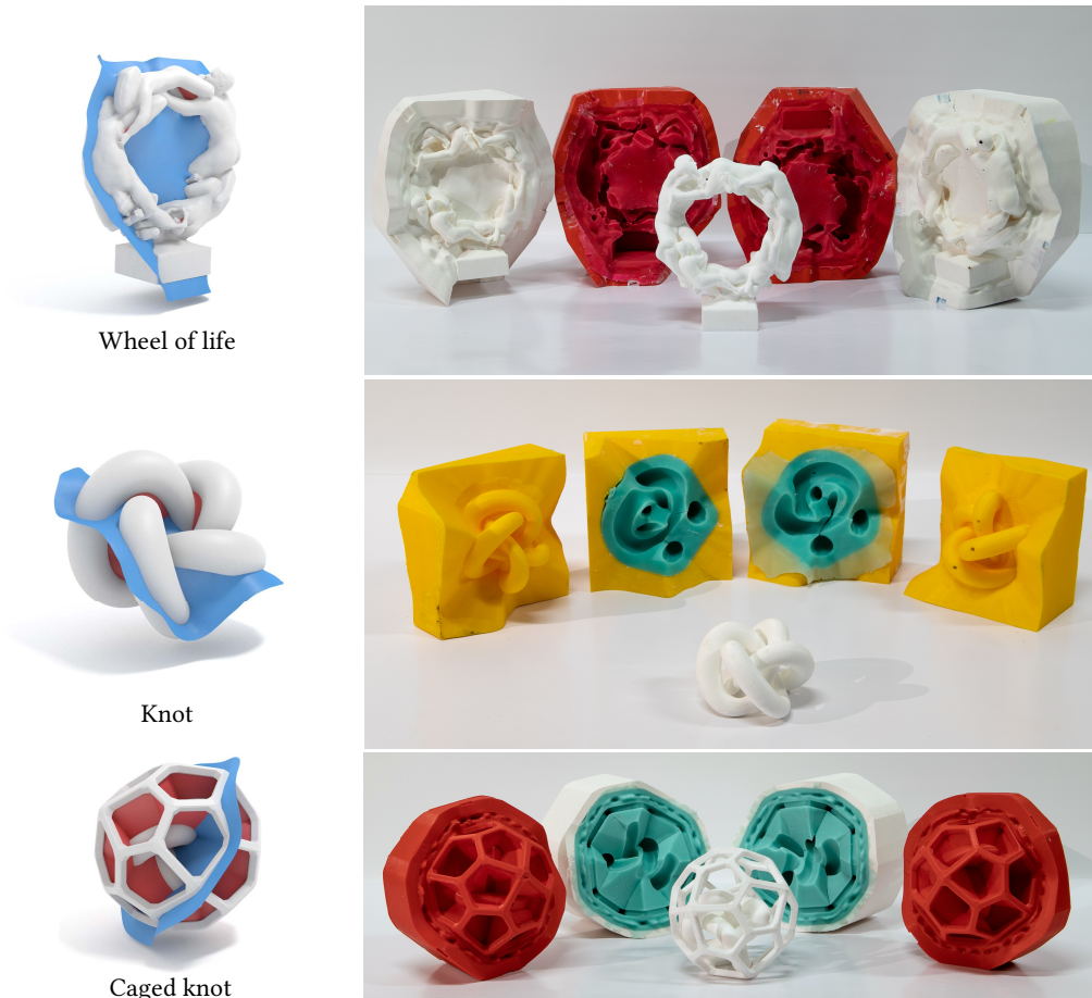
Fig. 14. Successful casting of a surface of non-zero genus, a knotted shape, and an object composed of two entangled pieces.
