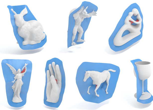
Fig. 17. Running our method on the dataset of Metamolds [Alderighi et al. 2018] always produces a valid set of membranes.
