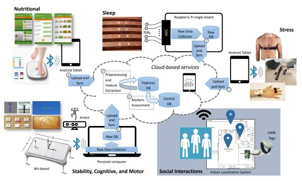
**Figure 1.** Overview of the deployed services with their devices, local gateways, cloud-based back-end modules.
