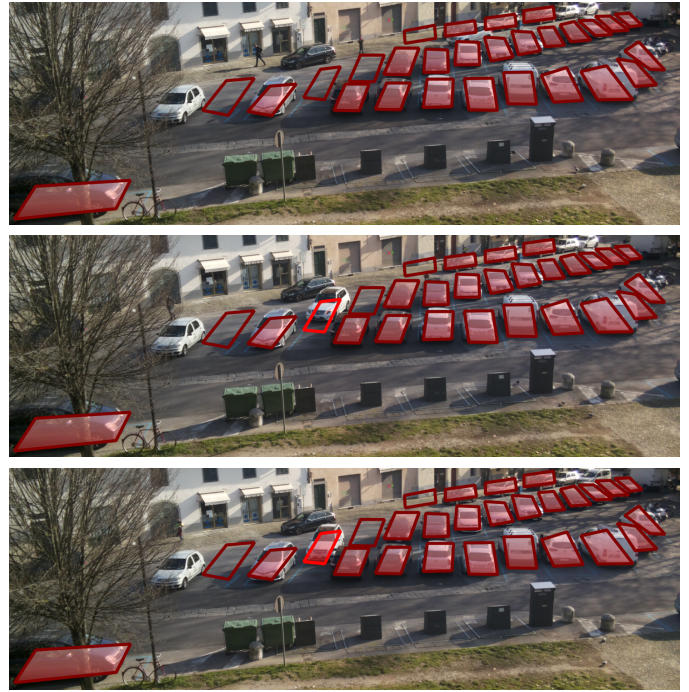
Fig. 6. Sample of three frames with a new detected vehicle entering and occupying an available space.
