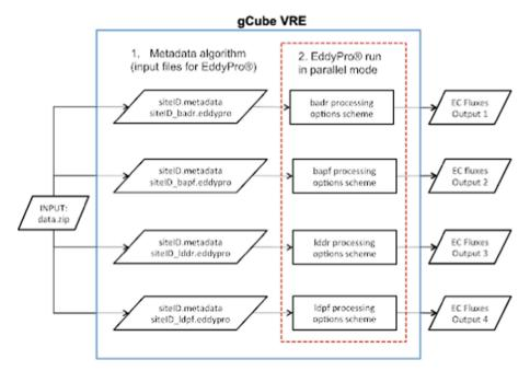
Fig. 5. EC data processing path.
