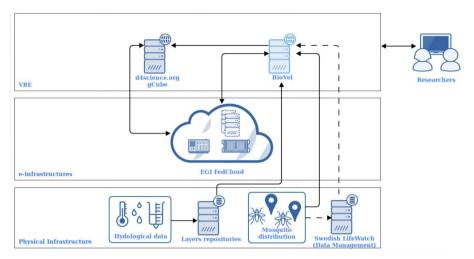
**Fig. 8.** Architecture includes three layers: 1) Physical Infrastructure, 2) e-Infrastructure, and 3) VRE.
