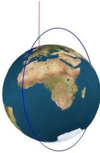
Figure 18: Intersection between the line connecting the ground station to the observed object position and the orbital plane
