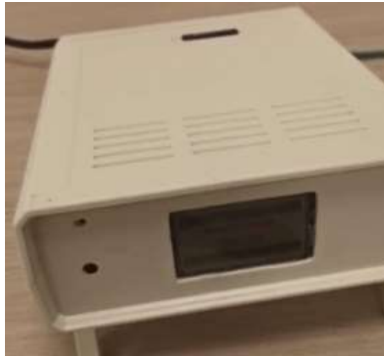
Figure 134: DS WOQ The uLive controller serving as gateway
