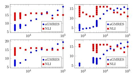
Fig. 5.5: Number of IPM iterations and average GMRES iterations during the IPA steps for the Poisson (left) and convection-diffusion (right) problems for FEM step-lengths  $h = 2^{-5}$  (top) and  $h = 2^{-6}$  (bottom) over the penalty parameter  $\varepsilon$ .
