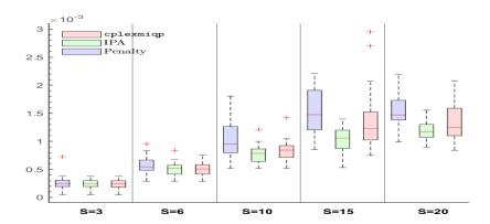
Fig. 5.3: Results of the second experiment: for each part of the test set, a boxplot related to the objective function of the final solutions attained by each algorithm is depicted. For S=10, 15, and 20 the boxplot for cplexmiqp is plotted with respect to the right y-axis.
