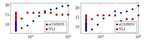
Fig. 6.2: Number of IPM iterations and average GMRES iterations during the IPA steps for the nonlinear problem instance for FEM step-lengths  $h = 2^{-5}$  (left) and  $h = 2^{-6}$  (right) over the penalty parameter  $\varepsilon$ .
