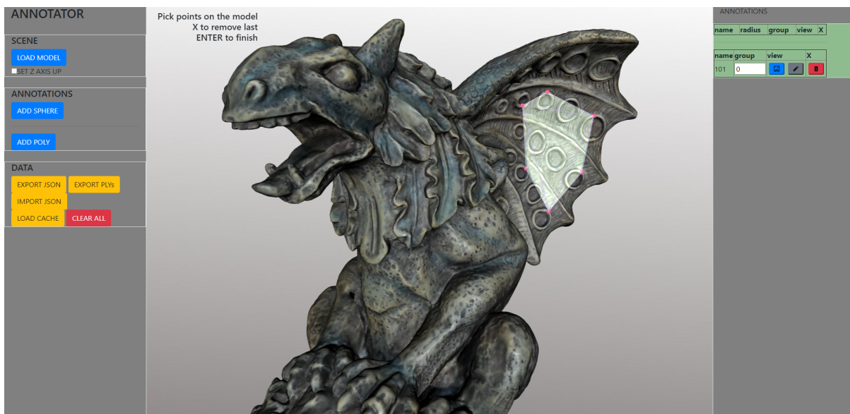
Figure 4: The experimental version of the polyline-based annotation service. The panel on the left contains the button for adding the polyline hotspots (in light green) in the 3D scene. Through the panel on the right is possible to modify the hotspot setup (groups ID, associated view), as well as remove them.
