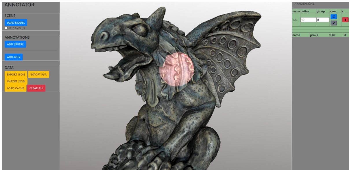
Figure 3: The beta version of the sphere-based annotation service. The panel on the left contains the button for adding the sphere hotspots (in light pink) in the 3D scene. Through the panel on the right is possible to modify the hotspot setup (radius, groups ID).
