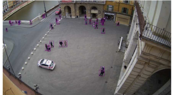
Figure 2: A sample from our novel CrowdVisorPisa dataset, together with bounding box annotations localizing pedestrians.
