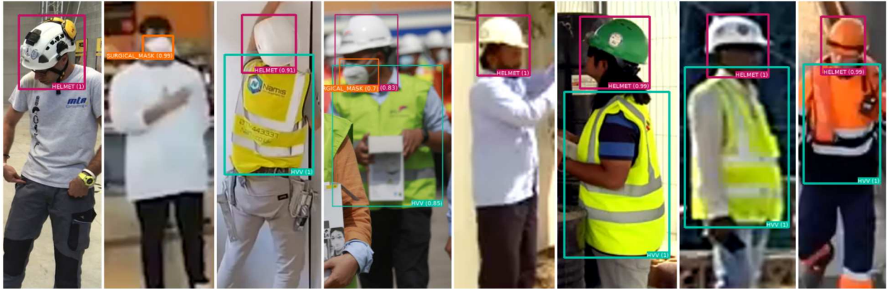
Figure 7: Examples of predictions of the PPE Detection module on our CrowdVisorPPE test set. PPE classes are color coded ( helmet , high-visibility vest , face mask ), and the detection score is reported in parenthesis.
