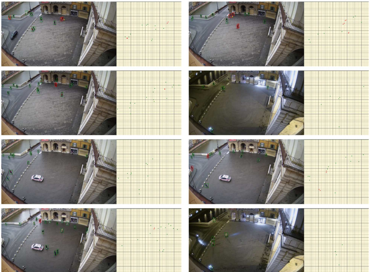
Figure 8: Examples of detections and distance warnings under different lighting conditions. Each of the eight images represents, in its left side, pedestrians detected and tracked in the example scenario, while showing on its right side their 2D projection on a virtual planar surface obtained through homography, with a reference 1-meter-spacing overlay grid. Green color means a safe placement, red color indicates violations of the 1-meter physical distance rule.
