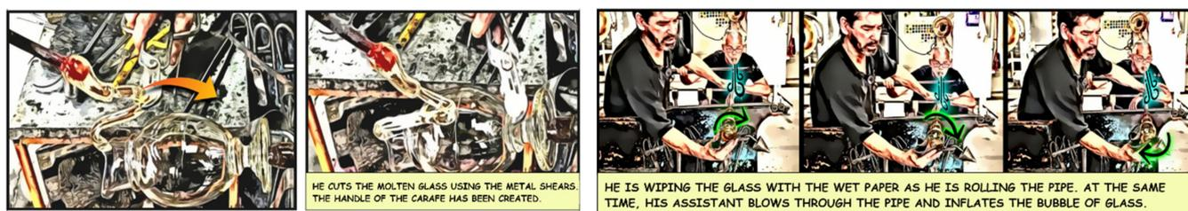
**Figure 14.** Illustrated demonstration of glassblowing.
