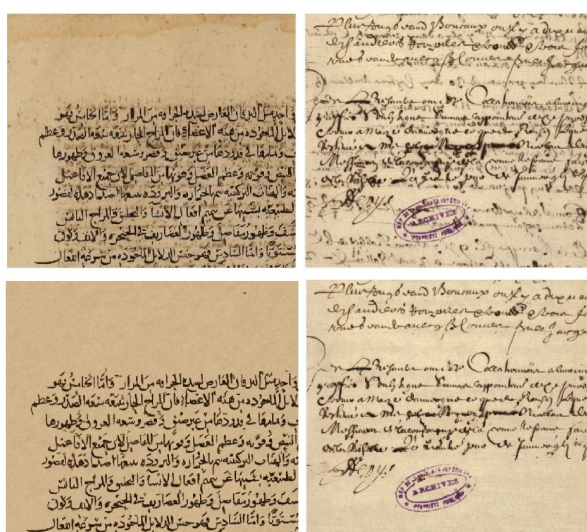
Figure 4: Visual examples of ancient document image restoration: input image (top row), restored image using the proposed method (bottom row).
