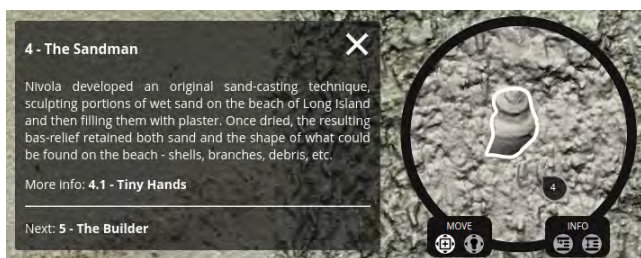
Figure 12: The interactive lens. The lens is the central interactive object. By moving and scaling it, the view is also automatically controlled. Buttons that decorate the border give access to lighting and annotation navigation control. The information area describes the current annotation, following the lens. Interactive and decoration areas are only visible when the lens is steady.
