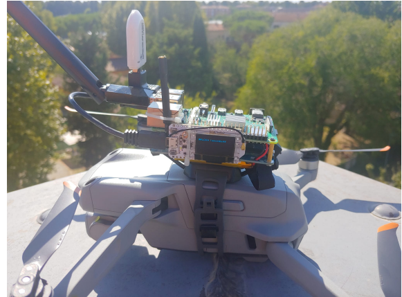
Fig. 2. The OnBoard node installed on a commercial drone
