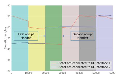
Figure 3. Elevation angles of the pair of satellites connected to the UE in different contexts.
