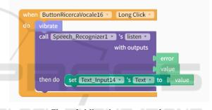
Figure 3: Microphone usage code.
