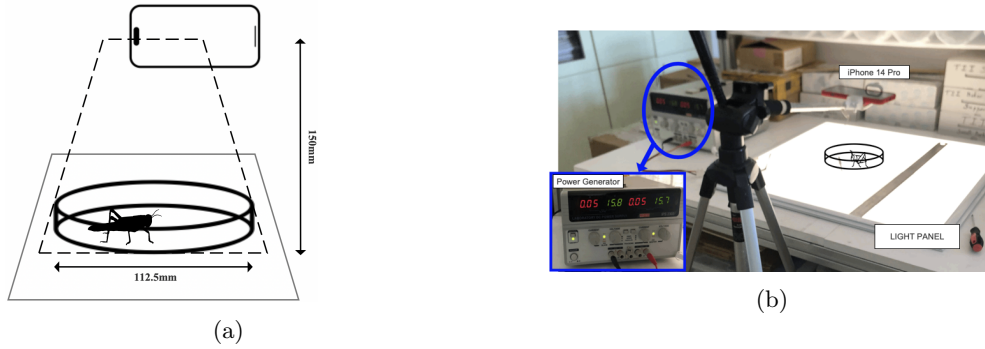
Fig. 1: (a) shows an illustration of the setup employed for recording the crickets. (b) shows the real setup in our lab.
