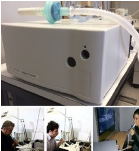
Figure 5: The e-nose device used to monitor severe liver impairment.
