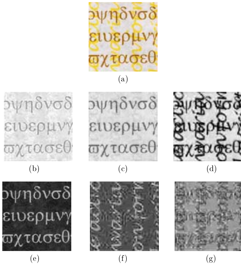
Figure 2: Synthetic example of a palimpsest: (a) color image; (b) red channel; (c) green channel; (d) blue channel; (e) first FastICA output; (f) second FastICA output; (g) third FastICA output.
