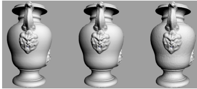
Figure 4.11: An example of good simplification. Even when the geometric complexity is greatly reduced, all the details are preserved. Left: 2.104.792 faces, Middle: 130.343 faces, Right: 19.936 faces
