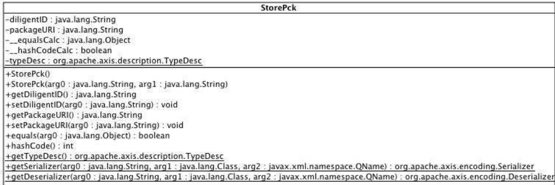
Figure 69. Package Repository: StorePck Class Diagram
