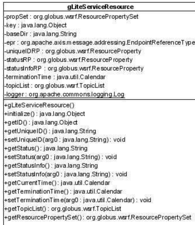
Figure 28. DIS-R-GMAClient: gLiteResource class diagram
