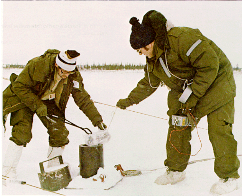
Radioactive debris being prepared for removal. In general, the materials were wrapped in plastic film to prevent dispersal of any dust or fine particles. The more radioactive objects were then manipulated into special shielded containers for safe transport.
