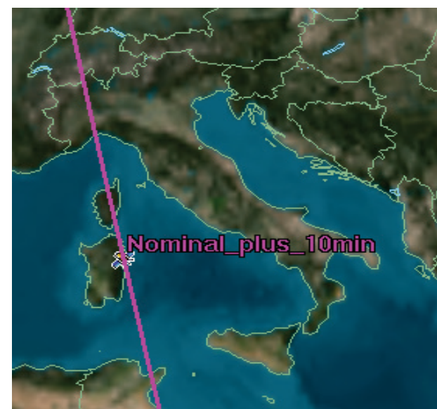
Westward drift of the sub-satellite ground track over Italy caused by an ascending nodal crossing delayed by 10 minutes
