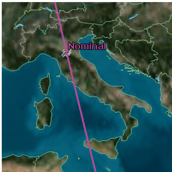
Predicted sub-satellite ground track over Italy of a re-entering satellite in nearly circular orbit at sun-synchronous inclination
