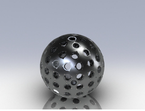
Fig. 2. A rendering of the LARES satellite. LARES is made of a unique piece of tungsten (THA-18N, composition 95% of W and 5% of Cu and Ni) and its surface is covered with 92 CCRs for SLR tracking. The CCRs mounting system is quite similar to that of the two LAGEOS. The satellite radius is 18.2 cm and its mass is about 386.8 kg. The area-to-mass ratio is about a factor of three smaller than that of the two LAGEOS satellites. Indeed, LARES is the densest object ever launched by the man in space. The satellite orbit is almost circular with a semi-major axis of about 7820 km (corresponding to an orbital period of about 6883 s). LARES has been launched with the qualification flight of the new European launcher VEGA. We refer to [14], [15] for further details.
