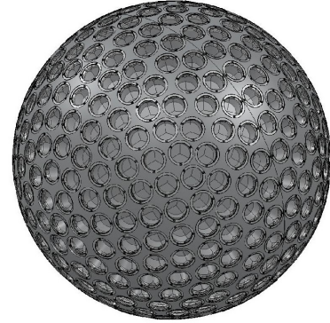
(b) Model of LAGEOS II at the finite elements
