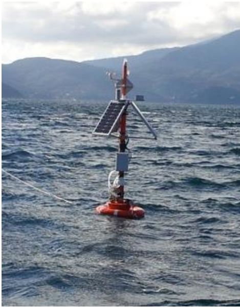
Fig. 1. The developed moored buoy at sea
