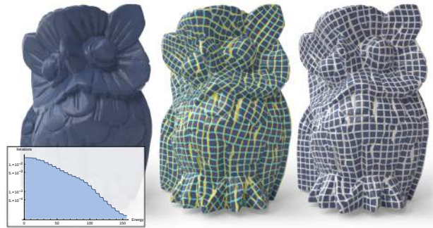
Figure 20: The Owl dataset (left), a 4-PoS computed using a 2-RoS (middle) and a 4-RoS (right). Bottom left: visualization of our extrinsic energy function for the result on the right. The steps through the hierarchy lead to a visible staircase pattern.
