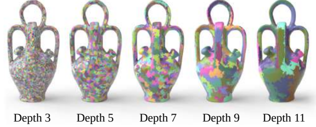
Figure 9: Our multiresolution hierarchy is created by merging adjacent vertices in the input graph in approximately \log_2 |\mathcal{V}| phases until only a single “super-vertex” is left per connected component.
