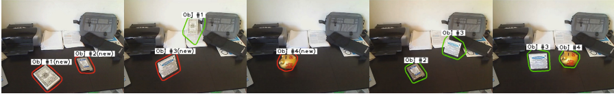
Fig. 6. Object learning and recognition in a test video sequence: objects are added, moved and removed from the scene. The system segments objects from the background and incrementally creates clusters of similar object views. An object is recognized assessing the membership of its current view to a pre-existent cluster.
